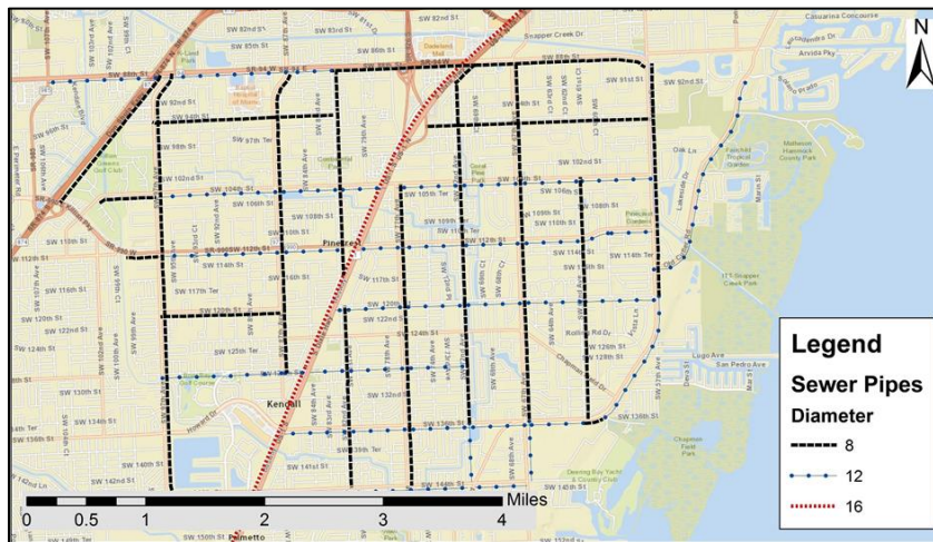
b. Sewer pipes diameter
