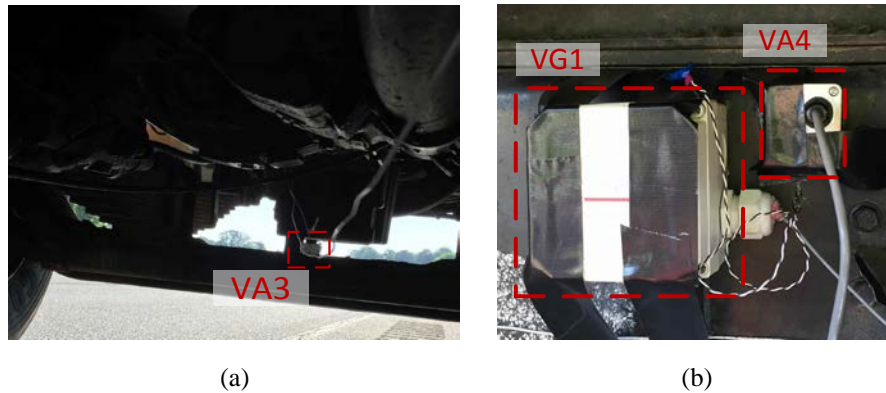
FIGURE 3-3 Installation of wireless sensors on the inspection vehicle: (a) accelerometer installed on the front axle; (b) accelerometer and gyroscope installed on the truck body
