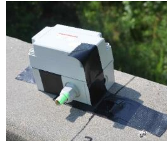
FIGURE 2-3 Truck position sensor: (a) laser emitter; (b) laser receiver; (c) instrumentation plan; (d) laser receiver installed on the bridge
