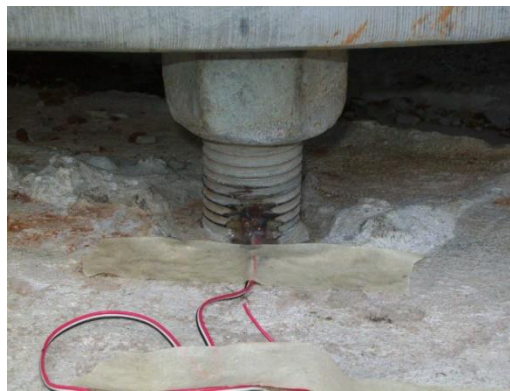
Figure 1.3 Uniaxial strain gauge mounted on an anchor bolt (Fouad et al. 2009)
