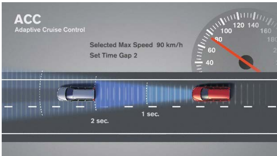
Figure 2. Adaptive Cruise Control Showing Selected Maximum Speed and Time Gap Setting (Johnson, 2012)
