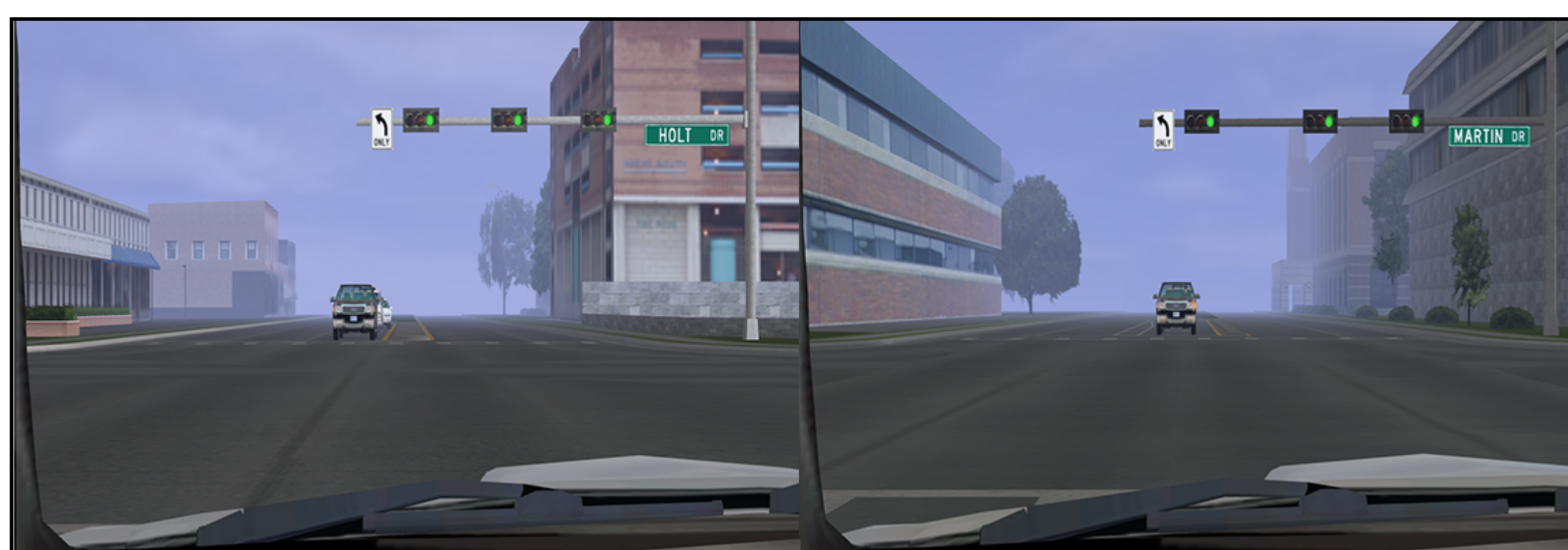
Figure 2. Driver's view from the left-turn lane for negative offset (left) and minimal negative offset (right) lanes
